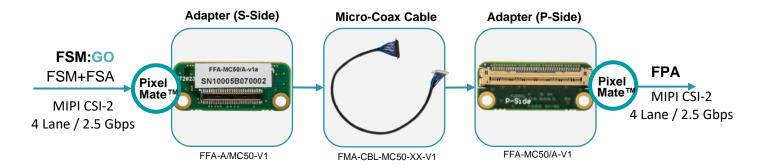
The components in this kit are passive and do not affect functional or software operations.
