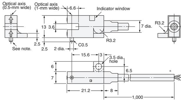
\* Vinyl-insulated round cable of 3.5 dia., 3 cores, (0.14 mm<sup>2</sup> with 1.0-dia. insulator); Standard length: 1 m
