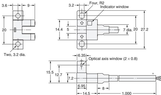
\* Vinyl-insulated round cable of 3.5 dia., 3 cores, (0.14 mm<sup>2</sup> with 1.0-dia. insulator); Standard length: 1 m
