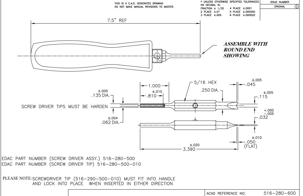
DATE: SEP.24/11 DRAWN: N.SONDH 516 CONTACT INSERTION TOOL CHECKED: DATE: SCALE: (IN C.A.D. 1:1) SHEET 1 OF 1 THESE DRAWINGS AND SPECIFICATIONS EDAC INC ARE THE PROPERTY OF EDAC INC., AND TORONTO, ONTARIO SHALL NOT BE REPRODUCED, OR COPIED DRAWING NUMBER **ISSUE** OR USED AS THE BASIS FOR THE CANADA MANUFACTURE OR SALE OF APPARATUS 516-280-600 YOUR CONNECTION TO QUALITY & SERVICE WITHOUT WRITTEN PERMISSION.
