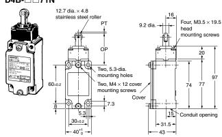
Note: Omitted dimensions are the same as those for the Roller Lever Type Models. D4B-1□□□N and D4B-5□□□N have a PG13.5 conduit opening. D4B-2 \Boxed \Boxed N and D4B-6 \Boxed \Boxed N have a G1/2 conduit opening. D4B-3□□□N and D4B-7□□□N have a 1/2-14NPT conduit opening
