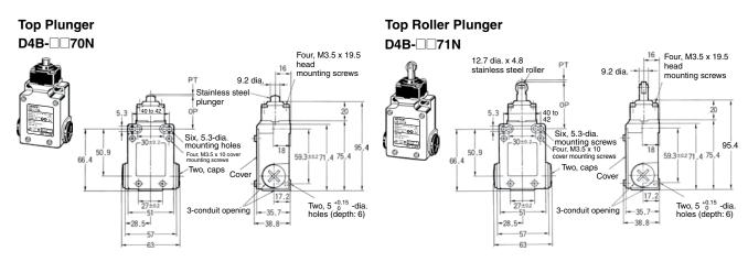
Note: Unless otherwise specified, a tolerance of ±0.4 mm applies to all dimensions.
