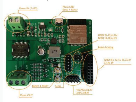
**Microcontroller**: ESP32 dual core, 240 Mhz, 4 Mb flash **Wi-Fi**: 802.11 b/g/n/d/e/i/k/r (802.11 n up to 150 Mbps) **Bluetooth**: v 4.2 BR/EDR and BLE specification
