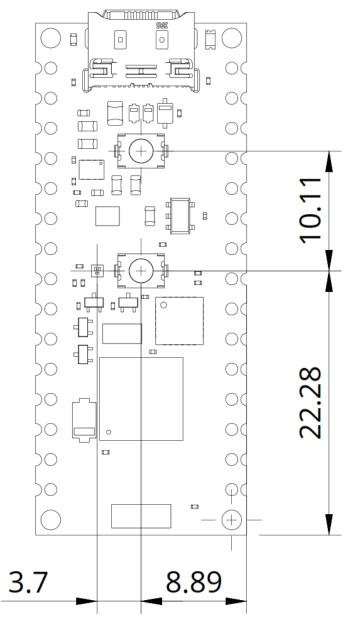
The Nano Matter is designed to be usable as a surface-mount module and presents a dual inline package (DIP) format with the Nano-styled header connectors on a 2.54 mm pitch grid with 1 mm holes.
