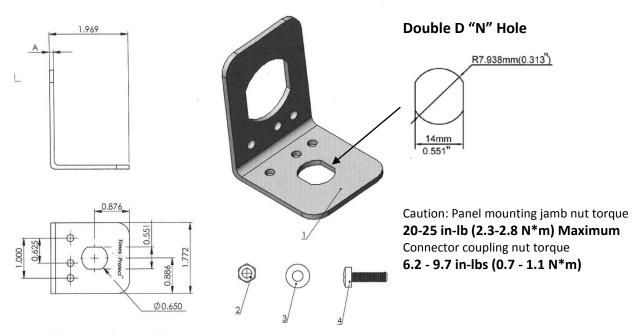
Drill (2) 4.8mm (0.1874") holes in grounded plate using the bracket as template. Attach bracket to ground plate with (2) M4x15mm, flat-washers under bolt heads, and star-washers under nuts (hardware supplied with bracket). Insert protector in "double D" N type connector hole.
