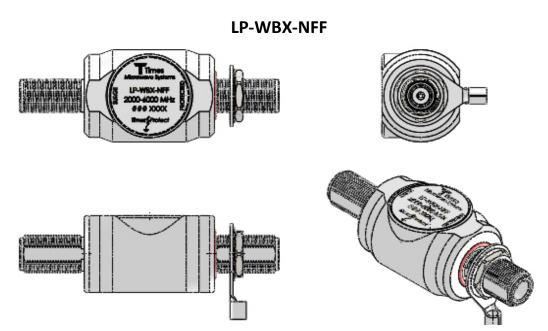
The LP-WBX-NFF and LP-WBX-NMP / NMS connectors are labeled "Surge" and "Protected". The "Surge" connector must be connected to the expected surge source (e.g. antenna). The "Protected" connector must be connected toward the protected equipment. *Protector failure and equipment damage can occur if the protector is installed backwards.*
