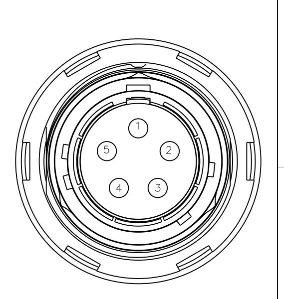
INSERT ARRANGEMENT 005A FIGURES SHOWN ASSEMBLED WITH KEY OPTION A
