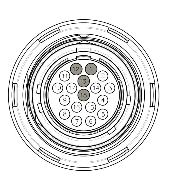
INSERT ARRANGEMENT 018A FIGURES SHOWN ASSEMBLED WITH KEY OPTION A
