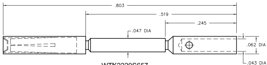
WTK2220S657 SOCKET, CRIMP REMOVABLE, 20 GAGE BARREL
