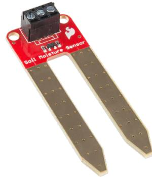
The VCC and GND pins are connected to an Arduino-based device (or compatible development board) to get the SparkFun Soil Moisture Sensor functioning. The user will receive a SIG out, which will depend on the amount of water in the soil. SparkFun have had PCB coated in gold finishing (ENIG, or Electroless Nickel Immersion Gold) to combat short lifespan of the soil moisture sensor when exposed to a moist environment.
