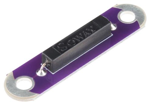
A reed switch is a simple mechanical switch that is activated via a magnet. When the device is exposed to a magnetic field, the two ferrous materials (reeds) inside the switch pull together, and the switch closes. When the magnetic field is removed, the reeds separate, and the switch opens. This makes for a great non-contact switch that can carry up to 1A and 0.25A while switched.
