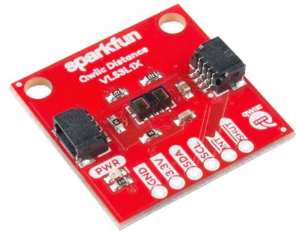
The VL53L1X ToF sensor uses a Vertical Cavity Surface Emitting Laser (VCSEL) that emits an IR laser to time the reflection to the target. This VL53L1X sensor measures the distance to an object from 40mm to 4m away with millimeter resolution. The VL53L1X ToF sensor features 1mm precision with an accuracy of around  $\pm 5$ mm and minimum read distance of 4cm.
