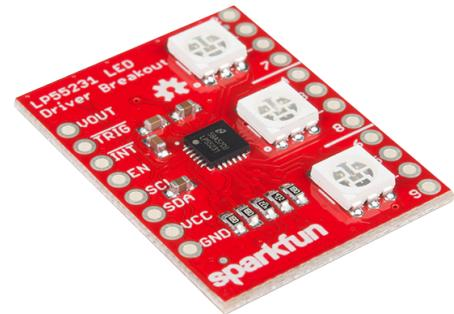
This breakout board drives LEDs using Pulse Width Modulation (PWM), so it's well-suited for variable intensity and color-mixing applications. Originally designed to be used in mobile device and automotive applications, the LEDs aren't meant to be overwhelmingly bright, and have some unique qualities.
