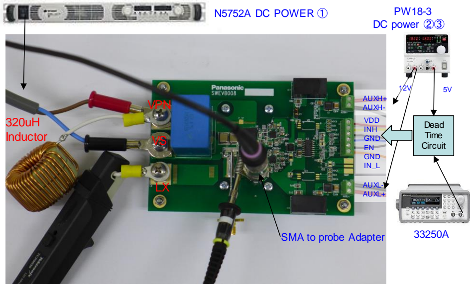
Figure 17: Connection for Low Side GaN testing
