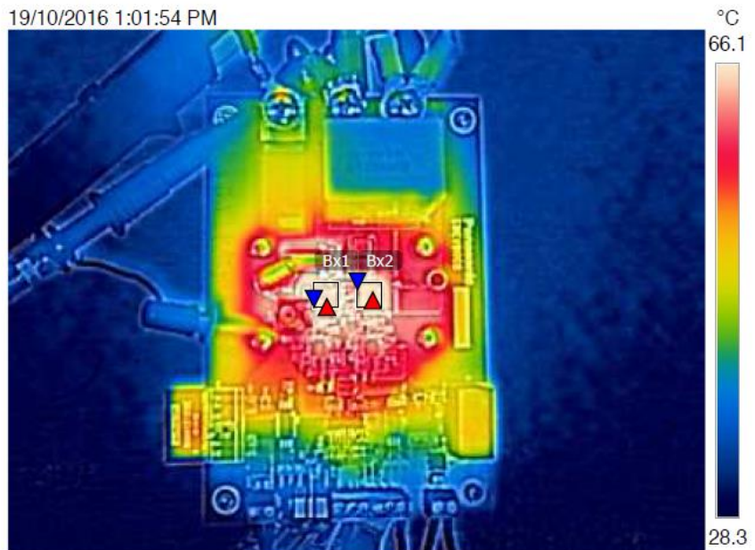
Figure 37: Thermal Profile of SWEVB008 in DCDC boost at 800W output power
