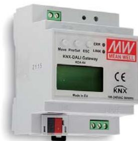
The device comes in a 4 unit's wide DIN Rail casing so it can be directly integrated into the mains distribution box. Connection to the KNX bus is via a standard KNX bus connector. Network and DALI lines are connected via screw terminals on the device.
