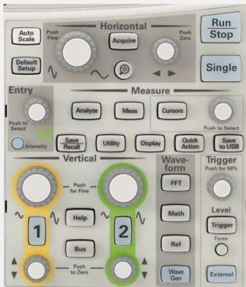
Figure 2. Oscilloscope front panels should include knobs for all key setup variables.
