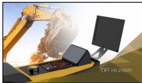
Touch Encoder supports no-look operations in off-highway vehicles.
