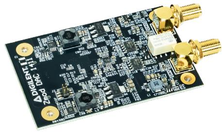
The analog outputs can be connected to a circuit using SMA cables. The combination of the SYZYGY expansion like Eclypse Z7 or Genesys ZU, when coupled with a baseboard, will serve as a powerful prototyping platform for instrumentation, high-speed control, and SDR. By utilizing these expansion capabilities, users can spend more time on the analytical and system-level aspects of the solution rather than focusing on the component-level interactions of the devices.
