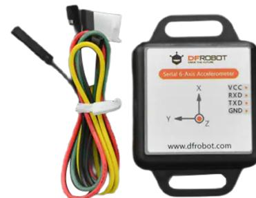
The serial 6-axis accelerometer module should be operated at 3.3V to 5V and the pin level is compatible with 3.3V/5V embedded systems. The 6-axis accelerator module employs TTL interface connection and supports adjustable 2400bps to 921600bps baud rate and 0.1Hz~200Hz data output.
