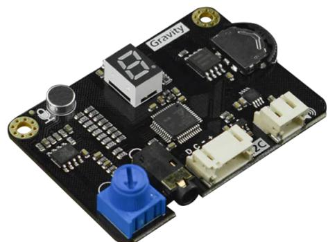
The gravity I<sup>2</sup>C voice recorder supports a number synthesis reading function, and simple programming can directly broadcast temperature, humidity, voltage, time, and other data. This module EDU also supports headphones or speaker output and built-in amplifier plug-and-play.
