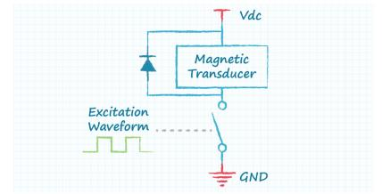
A magnetic transducer requires an excitation waveform to drive the buzzer. Arbitrary wave shapes and a wide range of frequencies can be used for the excitation waveform. The switch in the schematic is used to amplify the excitation waveform and is typically either a BJT or a FET. The diode is required to clamp the fly-back voltage created when the switch (transistor) is shut off quickly.
