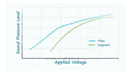
Figure 3: Graph showing the relationship between drive signal and audio output in piezo and magnetic buzzers
