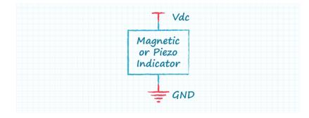
An indicator requires only a dc voltage to operate and sound is produced whenever the voltage is present.
