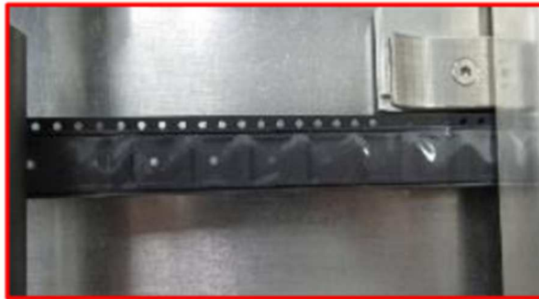
Carrier tape in taper with cover tape
