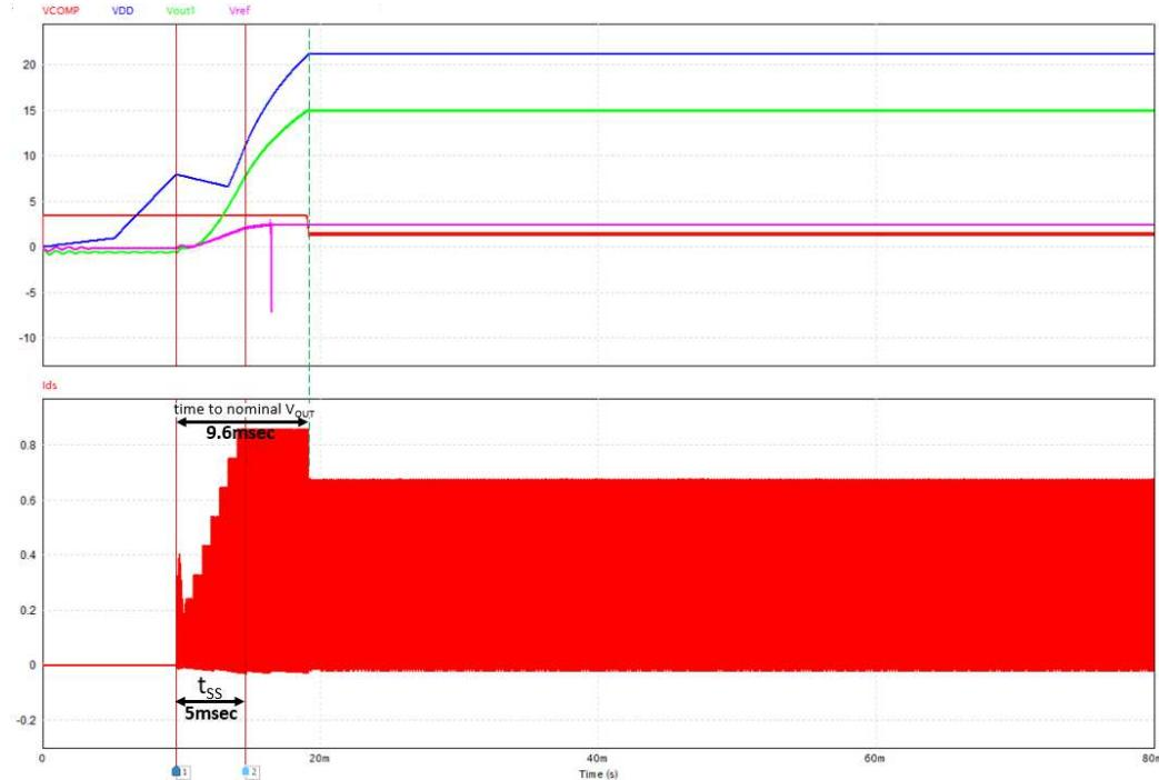
Result: if  $t_{SS\min}$  of «new range» is assumed in place of  $t_{SS\min}$  of «old range», the change we can expect in startup behavior is negligible
