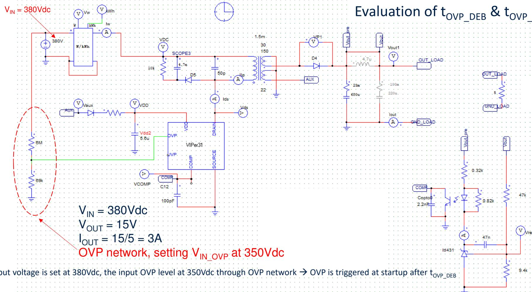
The input voltage is set at 380Vdc, the input OVP level at 350Vdc through OVP network  $\rightarrow$  OVP is triggered at startup after  $t_{OVP\_DEB}$
