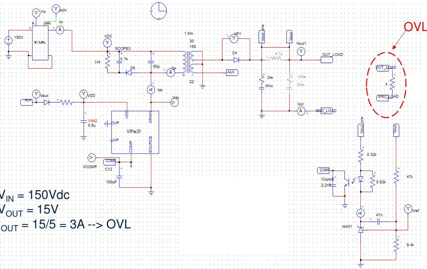
Output load has been set to 3A, which is beyond the maximum manageable by VIPer31, thus triggering overload protection.
