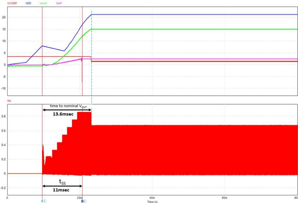
**Result: if  $t_{SS\max}$  of «new range» is assumed in place of  $t_{SS\max}$  of «old range», the change we can expect in startup behavior is negligible**
