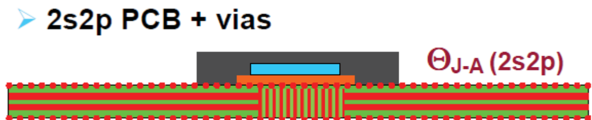
Figure 5. 2s2p PCB with thermal vias
