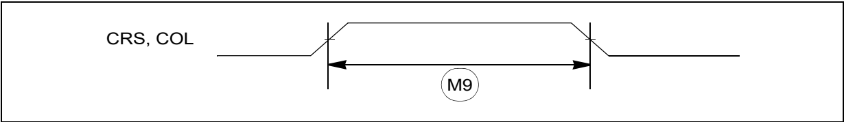
Figure 38. MII async inputs timing diagram
