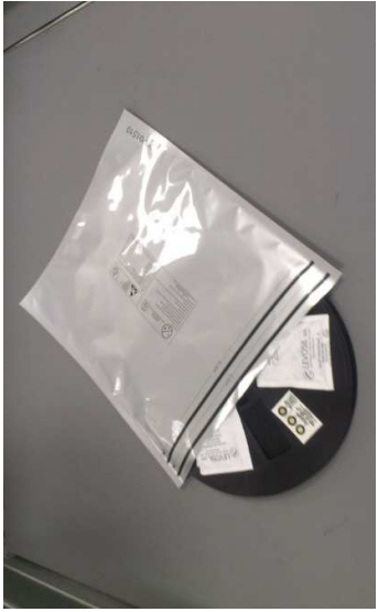
2 Desiccants and one Humidity Indicator Card in an ESD-safe Sealing Bag
