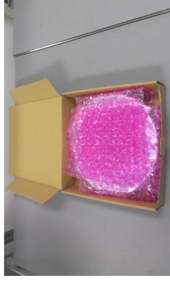
Bubble Wrap closed over Bagged Reel to increase impact protection
