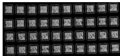
C-SAM (Reflected) @ Time-0 Results: No Delamination
