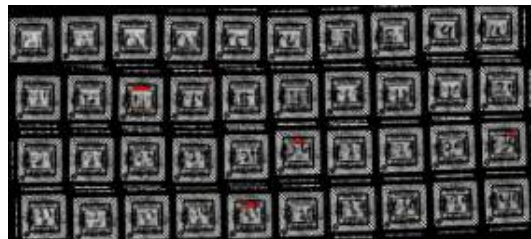
C-SAM (Reflected) After MSL3 (3IR) Results: No Delamination
