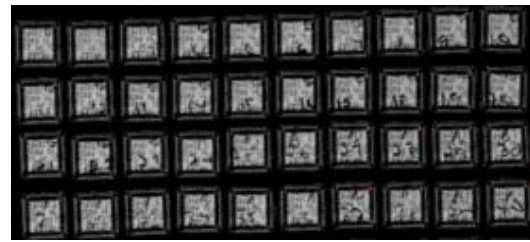
C-SAM (Reflected) @ Time-0 Results: No Delamination
