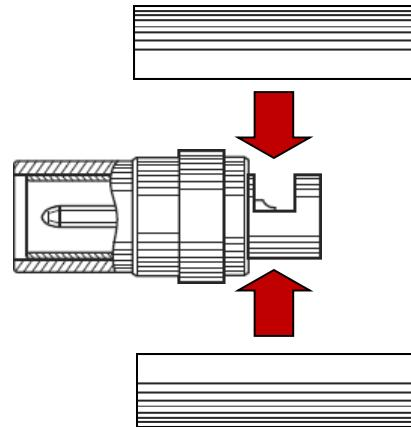
Triaxial inserts in the 1S, 1E, and 1V Series will now use a split insert carrier in cable mounted models like those used in the B and K Series.
