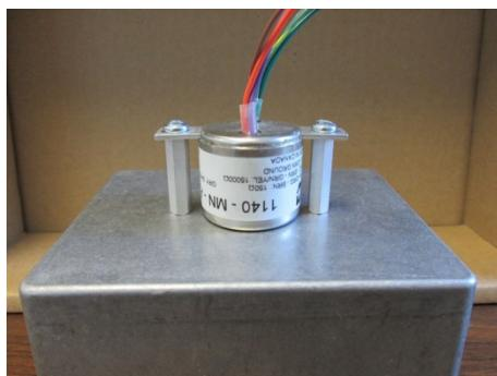
This last picture again is on the same enclosure but shows the leads going up and the mounting has the addition of 2 - 1.0" threaded standoff's to fasten the tabs to the enclosure
