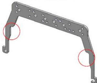
These two cuts improve handling and terminating modules for larger wires at the outer positions for the Han-Modular® Hinged Frame 24B size.
