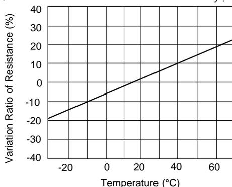
The variation ratio of the temperature coefficient will be comparatively larger with weak measuring light. The resistance value will increase as the ambient temperature goes up.
