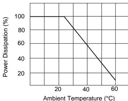
Tolerable power dissipation is the permissible amount of power the cell may dissipate when it is employed in a given circuit. This value is dependent on the characteristics of the photoconductive cell itself and is external covering in relation to ambient temperature and generated temperature all cells are measured at 25°C.
