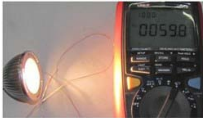
Figure 8: XP-E MR16 solder point temperature measurement
