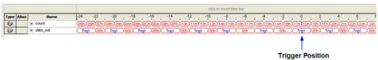
Figure 13-48: SignalTap II Logic Analyzer Continuous Data Capture
