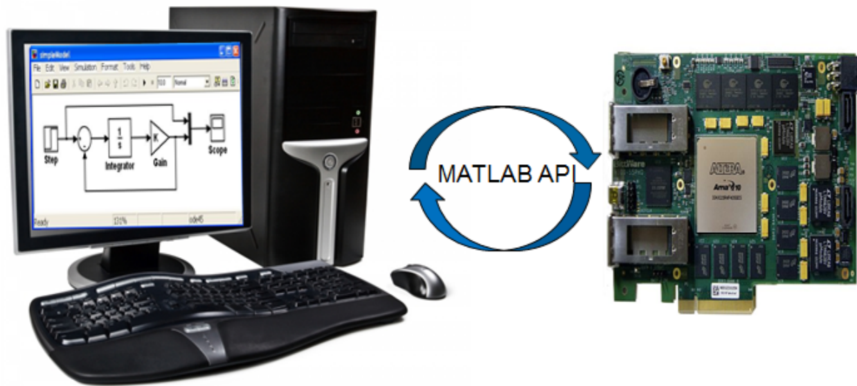
Figure 6-16: Hardware in the Loop Host-Target Setup
