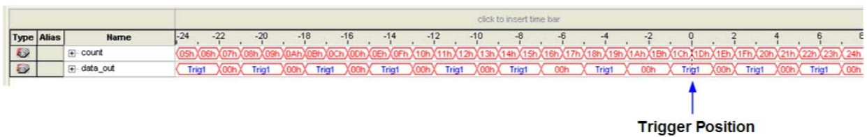
Figure 9-45: SignalTap II Logic Analyzer Continuous Data Capture
