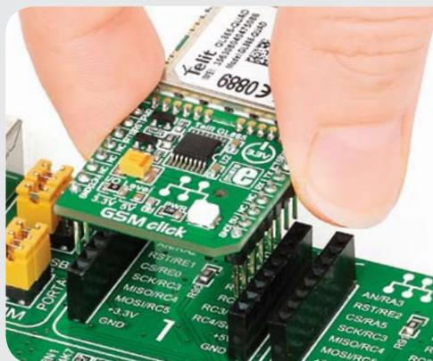
Once you have soldered the headers your board is ready to be placed into desired mikroBUS™ socket. Make sure to align the cut in the lower-right part of the board with the markings on the silkscreen at the mikroBUS™ socket. If all of the pins are aligned correctly, push the board all the way into the socket.
