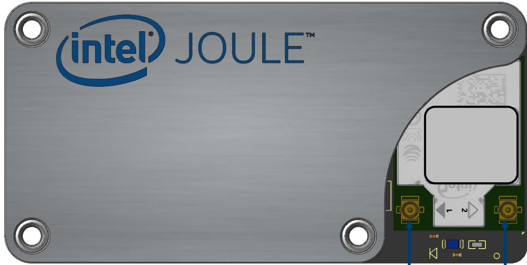
Antenna 1 Wi-Fi* only Antenna 2 Wi-Fi + Bluetooth* Antenna Connectors are MHF4 type
