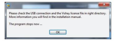
... please double check if the license files are in the correct place and the driver is installed, as described in the demo kit installation guide. Also make sure that the USB dongle and board are plugged in before you start the software.
