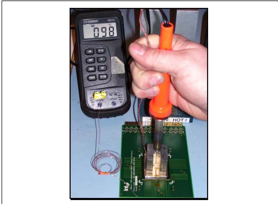
Figure 5-14. Observing the Solder Melting
