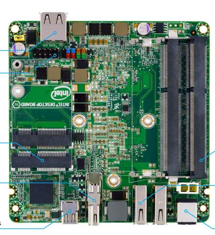
Dual channel SODIMM DDR3 1333/1600 MHz
