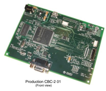
The CBC-2 includes a 33 conductor Flat Panel Cable (FPC) and screws to attach the PCBA to the LCD that exist in many 5.7" panels. The PCBA comes standard with the 33 pin connector stuffed. Optional, is a 31 pin header that can be stuffed (customer option) to support those displays using that style connector and signals.
