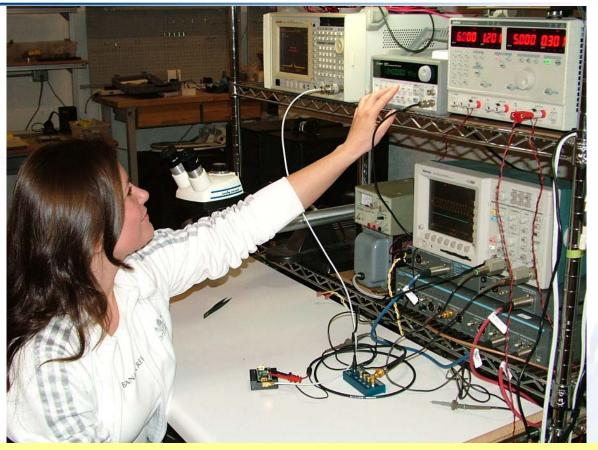
In this example, the ABPSM-ULN-A is being used to provide Ultra-Low-Noise Bias for an RF Amplifier. The output of this Amplifier is being measured for Spectral Content, using a Spectrum Analyzer.
