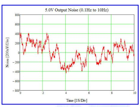
Similarly, both 3.30V & 5.00V bias ports exhibit better than +/-500nVp-p noise over 0.1Hz to 10Hz bandwidth.
