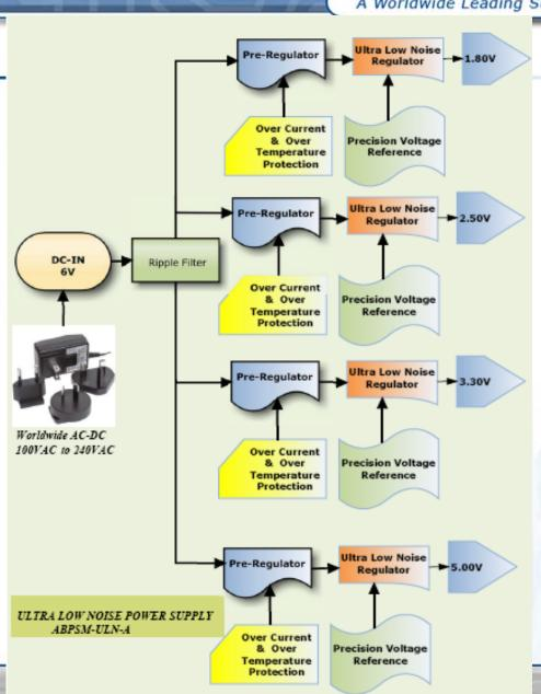
Overall design approach incorporates a Ripple Filter, followed by preregulation, regulation and precision voltage reference architecture. Over current and over temperature protection prevents any accidental damage to this device.
