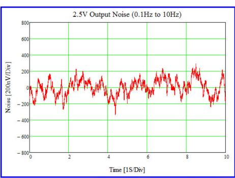
ABPSM-ULN-A offers exceptionally clean, low frequency noise characteristics. As is evident from the measured data, both 1.80V & 2.50V bias ports exhibit better than +/-400nVp-p noise over 0.1Hz to 10Hz bandwidth.
