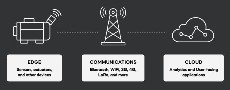
A large piece of the IoT architecture is the interface between the physical and digital world, the "edge". The "edge" consists of sensors and actuators that interact with the surrounding environment. Sensors take measurements and collect data, perform some analytics and machine learning, then transmit to the cloud where further global analytics and machine learning can present actionable insight. For IoT to be successful, edge devices need to provide the following:
