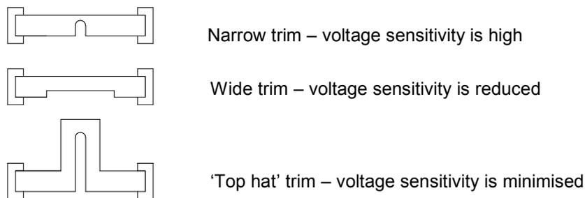
Figure 2d: VCR dependence on trimming geometry
