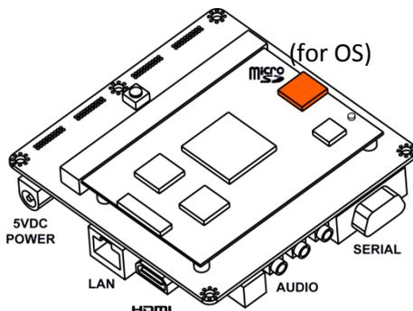
**f) Power up:** Plug in a power supply (5 VDC at 2A is recommended)
