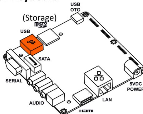
**e) Insert the microSD (orange microSD card slot)**
