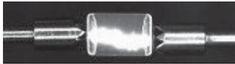
Standard Capacitor with Surface Arc-over
