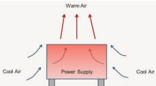
As the hot air rises, cooler air is drawn in from the sides. Although the airspeed is quite low, just 0.3m/s, it is sufficient to reduce internal temperatures. During the safety certification process for the power supply, this is taken into account during thermal testing.
