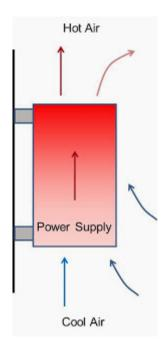
If in doubt, consult the manufacturer's installation manual. For high density products, recommended maximum component temperatures will be advised for critical parts.
