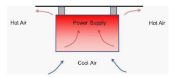
The ramifications of mounting the power supply vertically should also be studied. Ideally the input (bulk) and output electrolytic capacitors should be located at the bottom, where the temperature will be the coolest.
