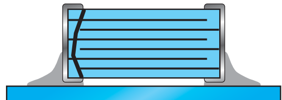
Type B: Fracture from top of device to bottom of device.
