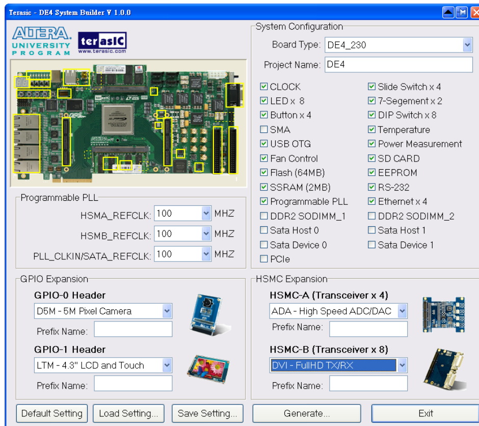
Figure 4-2 The DE4 System Builder window
