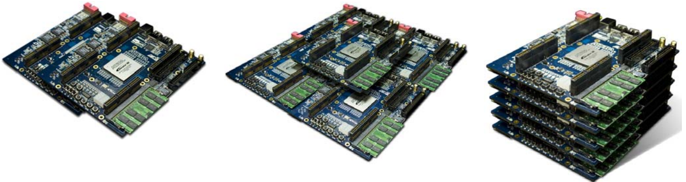
Figure 1.1 The stackable mechanism of the DE3 board
